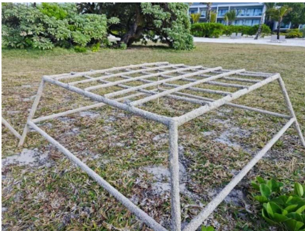
Figure 1. Refurbished spider frame prepared with resin and sand prior to deployment.
